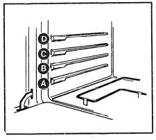
The oven has four shelf supports marked A (bottom), B, C and D (top). Shelf positions for cooking food are suggested on Baking, Roasting and Broiling pages.
